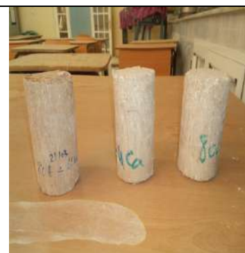
Figure .5. Tuff blocks reinforced with cardboard
