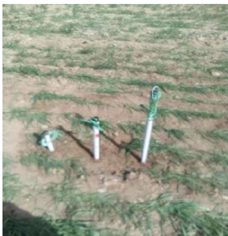
Figure 4. Tensiometers at different depths (0-20 cm/20-40cm and 40-60 cm)
