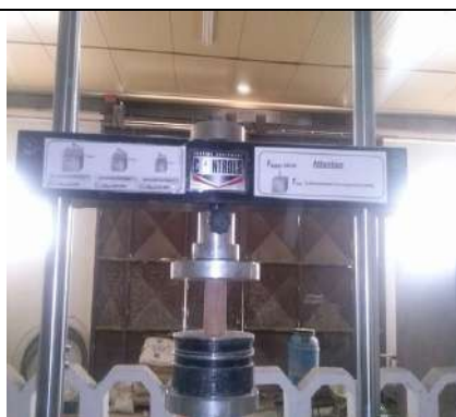
Figure .4. Press used for compacting and crushing test
