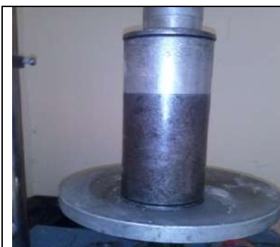
Figure .3 . Mould used for the manufacture of tuff blocks
