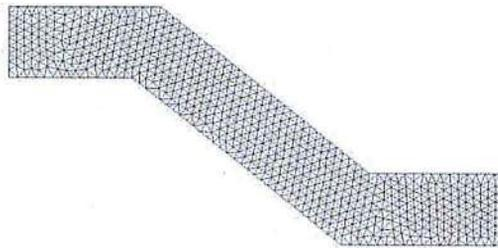
Fig 3. Mesh elements chosen for the simulations
